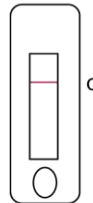
Negative: Only the quality control line (C) appears in the detection area.
